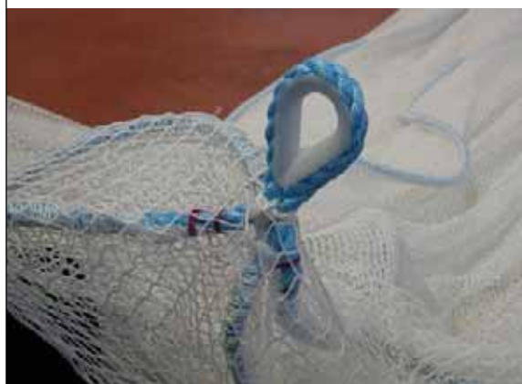
PLATE 65 Waterline rope loop with plastic thimble
