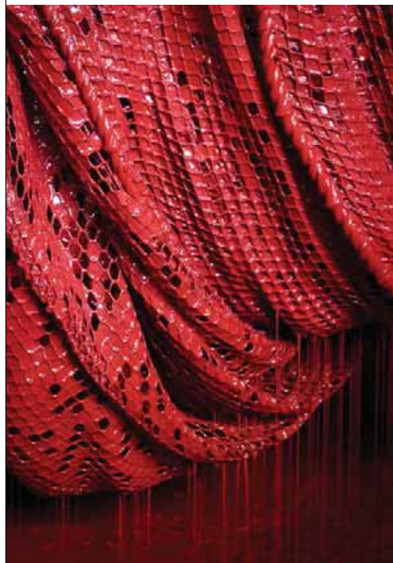
PLATE 78 Net dipping in an antifoulant tank
