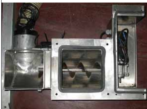
PLATE 106 The auger is installed below the hopper, where it moves the feed into the air duct (on the left)
