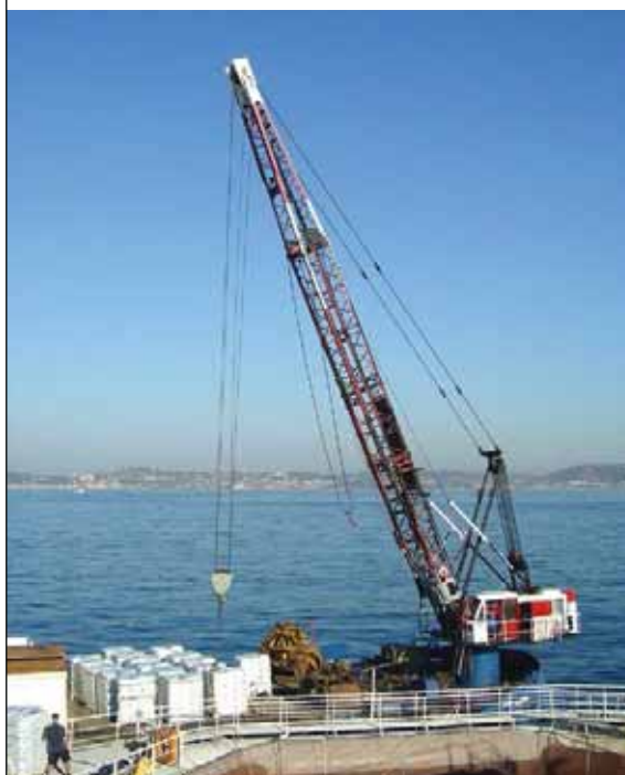
PLATE 103 A barge with a crane is used for handling of feed pallets
