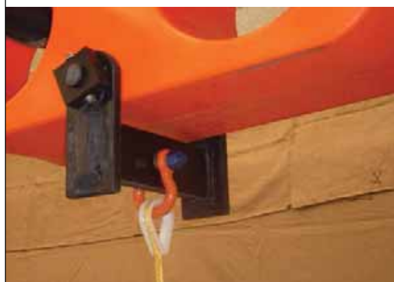
PLATE 38 Example of sinker rope connected to the base of the bracket
