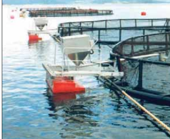
PLATE 113 Feed delivery pipes connecting the centralized feed system with the cages
