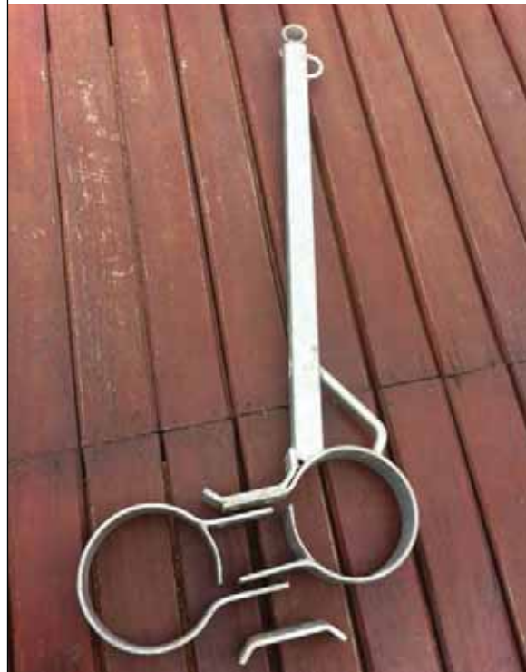
PLATE 28 Disassembled components of a galvanized steel bracket
