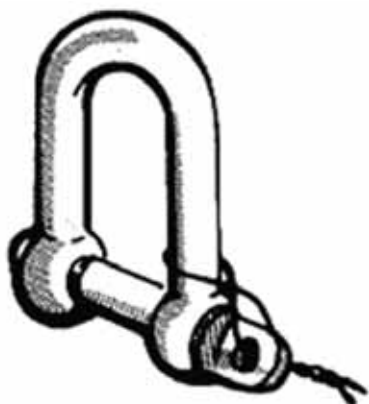
FIGURE 25 Shackles with clevis locked with a wire
