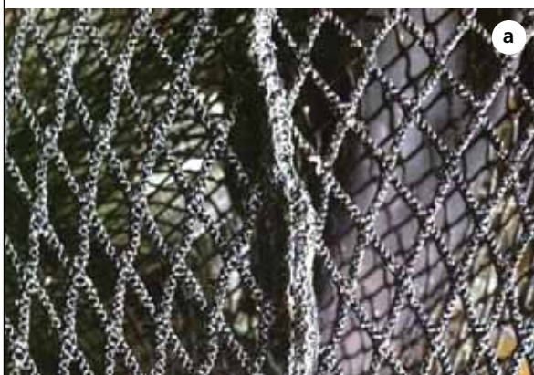
PLATE 55 Seams in cage nets. a) net to net; b) net to rope
