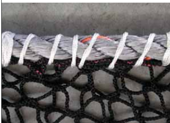
PLATE 58 Net to rope hand-sewn seam
