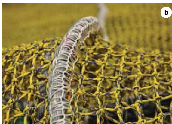
PLATE 55 Seams in cage nets. a) net to net; b) net to rope
