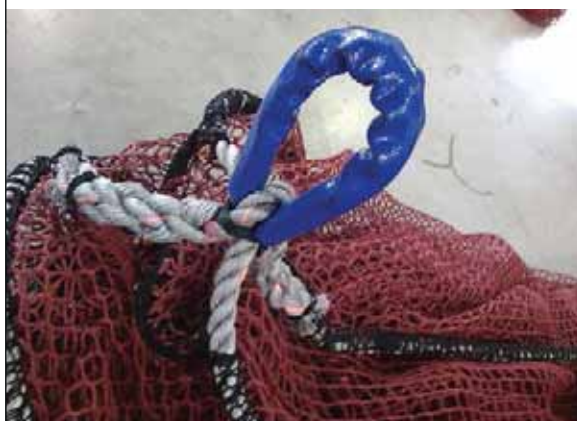
PLATE 64 Waterline rope loop with flexible pipe protection
