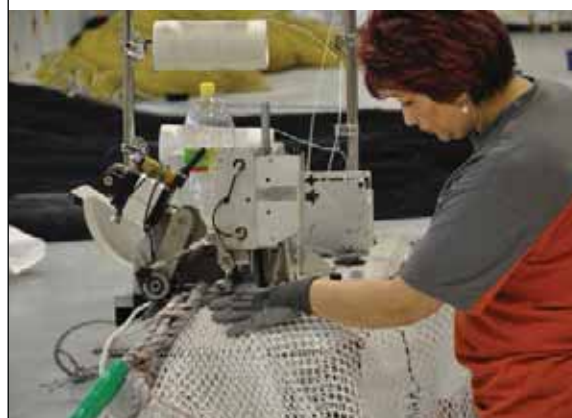
PLATE 57 Machine net to rope sewing
