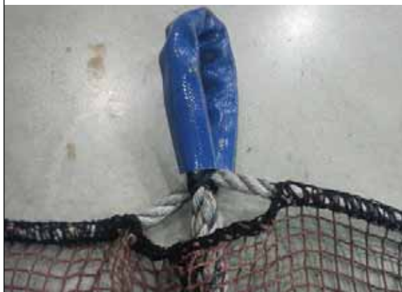
PLATE 62 Top rope loop, spliced with pipe protection
